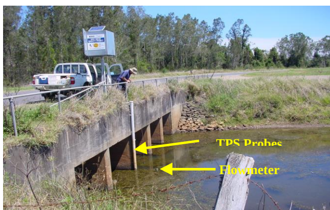
Plate 2.7 Location of TPS data logger probes and doppler at the discharge zone of Dungarubba Drain
